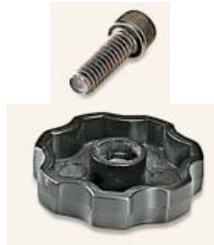
▲ Locking Knob. To make the locking knob for the layout square, a cap screw is press-fit into a blind hole in the center of the knob.
