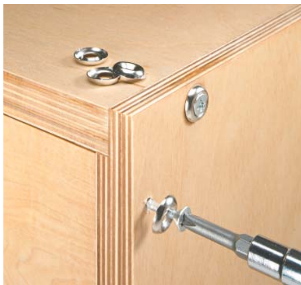
▲ Trim Washer. Trim washers are a great way to strengthen an assembly, especially near the edge where you may not want to countersink the screw.
