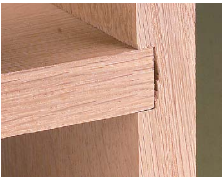
▲ Bad. A wobble dado set leaves a concave surface which can create large, unsightly gaps. Not only is this ugly, but the joint is not as strong.
