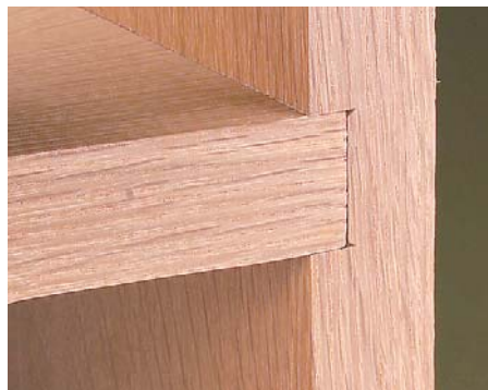
▲ Better. With stacked dado sets, the outside blades can leave score marks on the sides of the dado. While this doesn't weaken the joint, it's still noticeable.
