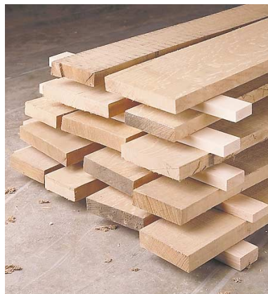
Let it sit. To let the wood adjust to the moisture level in your shop, stack boards with small strips in between.
