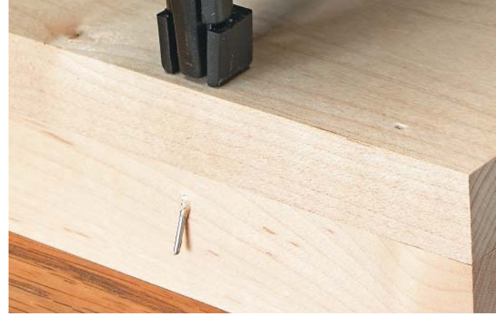
▲ As the pneumatic nailer is fired, the brad is sometimes deflected making the tip of the nail visible as it protrudes out the side of the workpiece.
