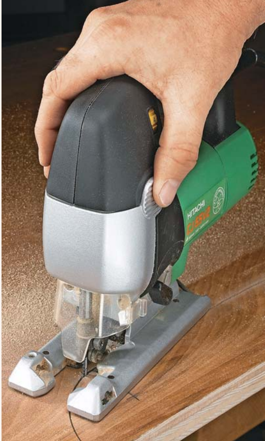
▲ Turn from the Front. Grip the saw directly above the blade when cutting curves. Take it slow, and let the blade do the work.
