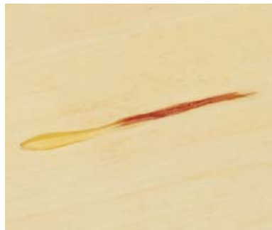
B. Pitch Pockets. These slits ooze sap which gums up saw blades and creates finishing problems.
