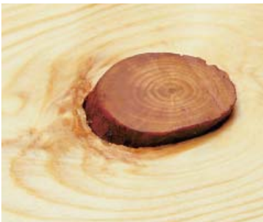
A. Loose Knots. A black ring around a knot is a sign that a knot will loosen up over time.
