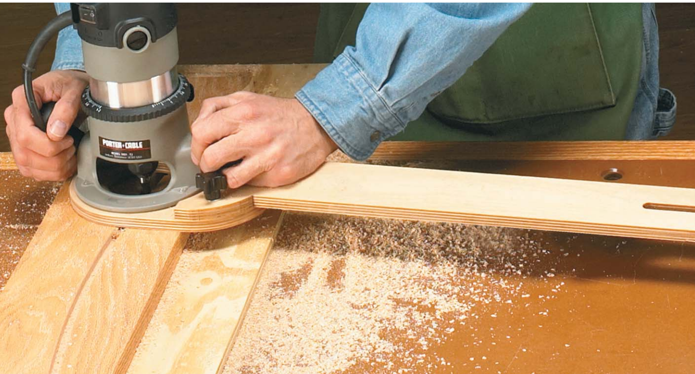
FIRST: CARPET TAPE WORKPIECE TO SCRAP PIECE, THEN CLAMP TO WORKBENCH
