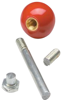
▲ Pivot Pin. All you need to make the pivot pin is a standard hex bolt and a threaded knob.
