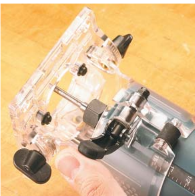
▲ Height Adjustment. You'll spend a lot of time adjusting the height of the bit. So you need to decide if you want the accuracy of a thumbscrew adjustment (left photo) or the speed of a quick-release lever (right photo).
