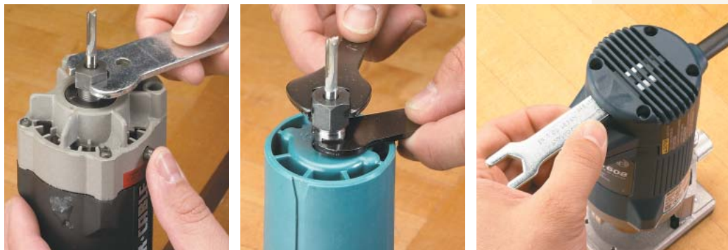
▲ Bit Changes. Like some full-size routers, trim routers that use a single wrench with a spindle lock are common (left photo). But trim routers with dual wrenches can be easier to use, whether both wrenches are used at the collet (center photo) or one slips into the top of the router (right photo).
