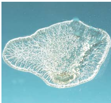
▲ A pure oil (tung or linseed) dries soft, wrinkled, and very slowly.
